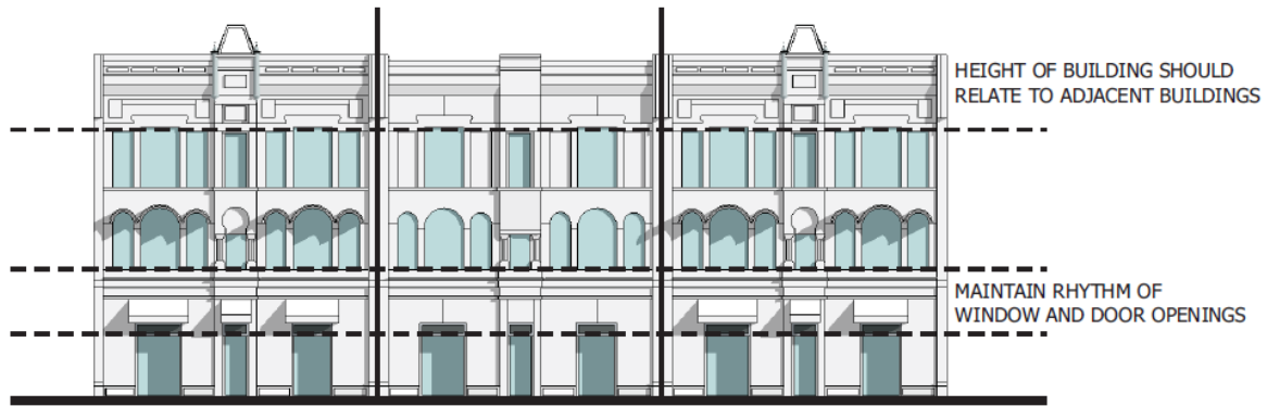
Figure 1110-D: The height, width, and overall proportions of infill development should be in scale with surrounding buildings. Buildings should also maintain the rhythm of window and door openings.
