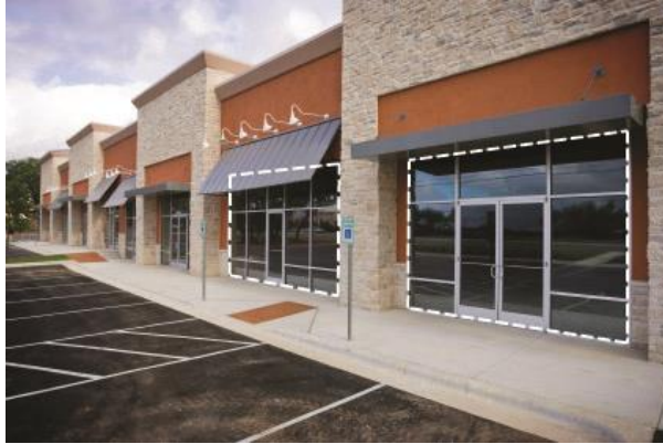
Figure 1113-M: The window area is illustrated within the dashed line area for the two storefronts in the above image.
