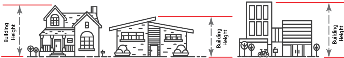
Figure 1105-K: Example of building height measurement.
