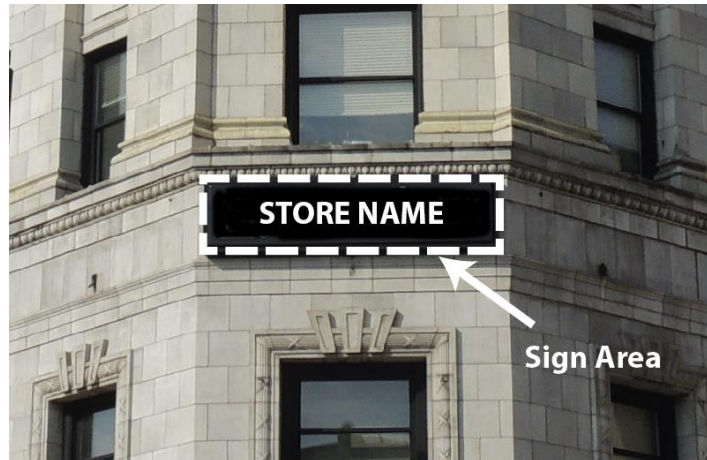
Figure 1113-E: Illustration of computing the sign area for wall signs with a background panel or cabinet.
