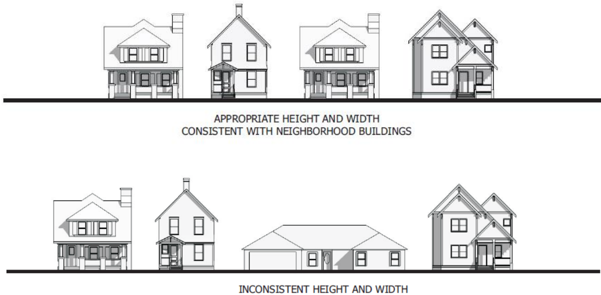
Figure 1106-A: The top image illustrates buildings that are constructed with appropriate heights and widths relative to the surrounding neighborhood whereas the bottom image illustrates a building that is inconsistent in height and scale.
