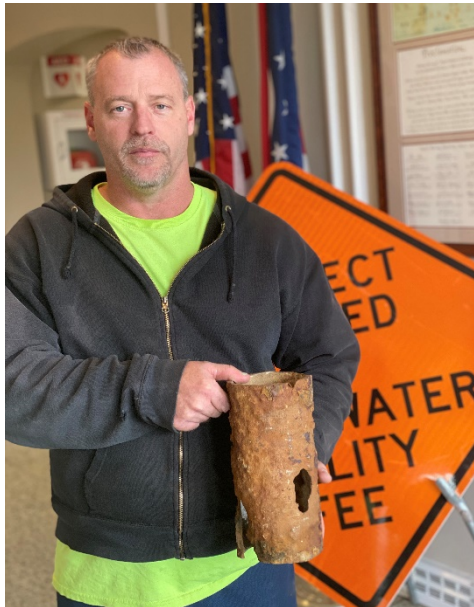
Jamie Pay, utility operations crew chief for the City of Mount Vernon's Utility Department, holds a piece of 70-year-old piece of cast iron pipe that was struck by lightning under East Chestnut Street on Aug. 12.
