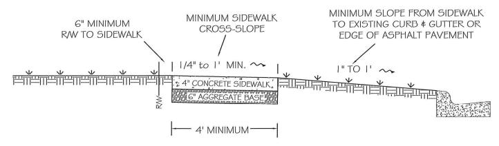
6" THICK MINIMUM AGGREGATE BASE REQUIRED (#8 OR #57)
